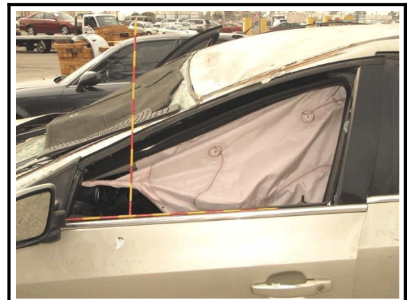
Figure 7. Deployed left IC air bag, area of coverage and tether location on A-pillar, 2015 Chevrolet Cruze
