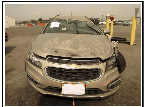
Figure 3. Front plane crush measurements, 2015 Chevrolet Cruze
