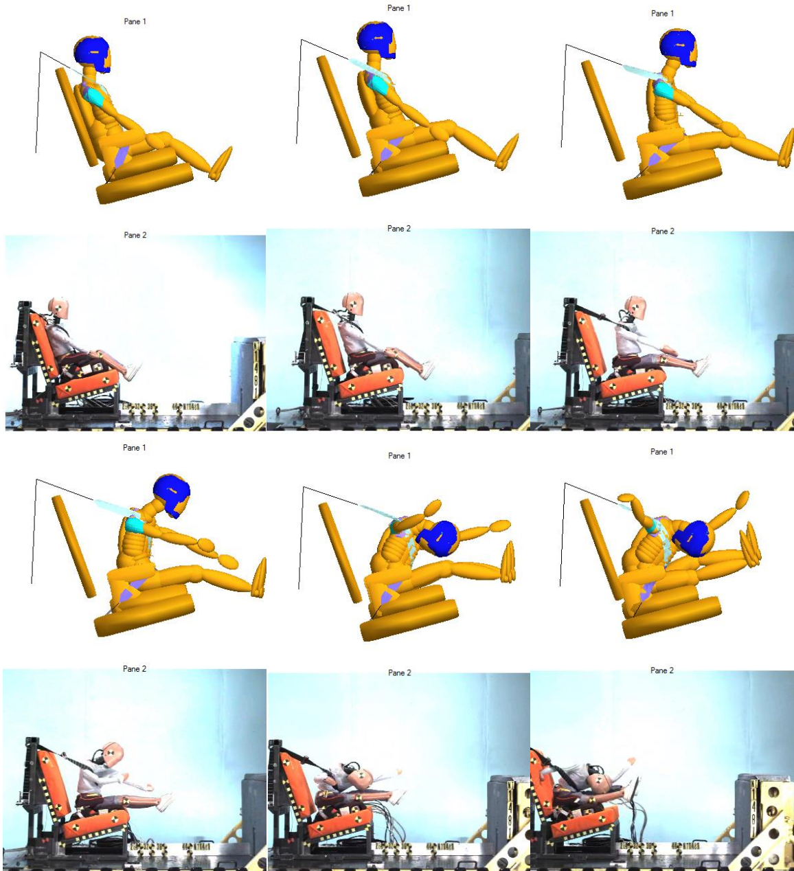
Figure 37. Kinematic comparison of model and test.
