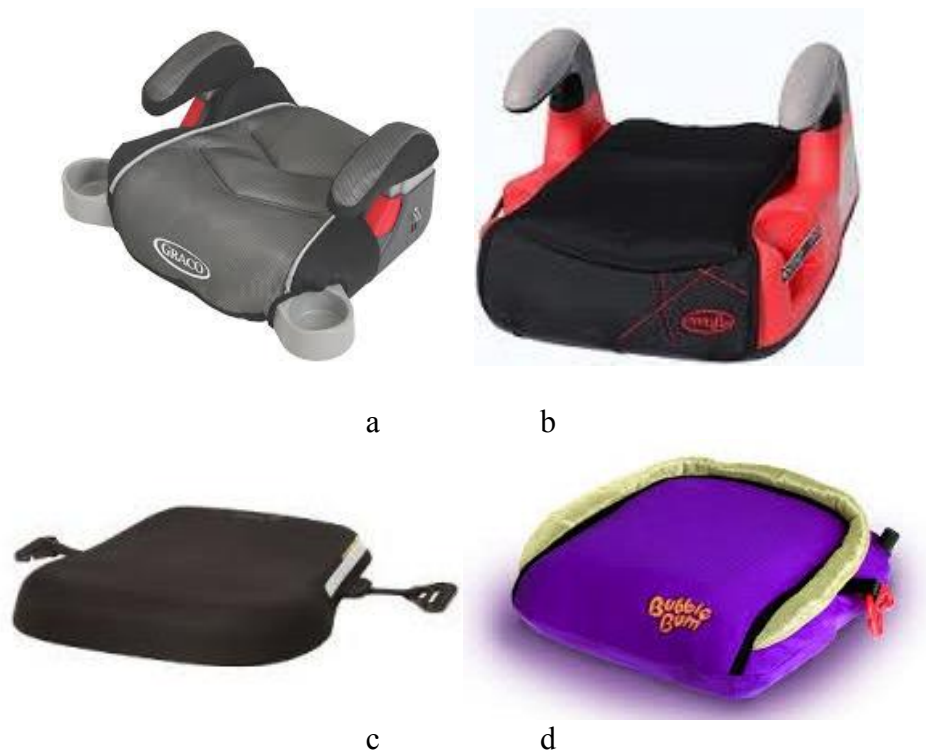
Figure 6. Booster seats used for testing: (a) TurboBooster, (b) Evenflo AMP, (c) Incognito, and (d) BubbleBum.
