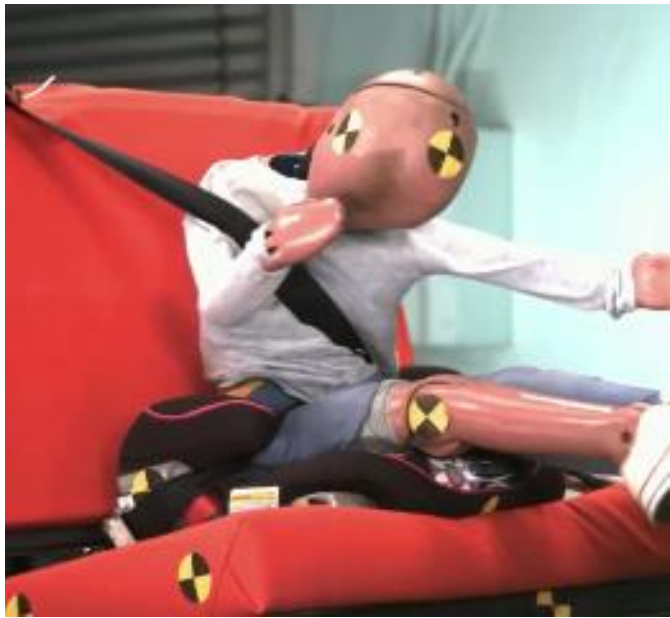
Figure 18. Example of ATD rolling out of the shoulder belt (NT1478).
