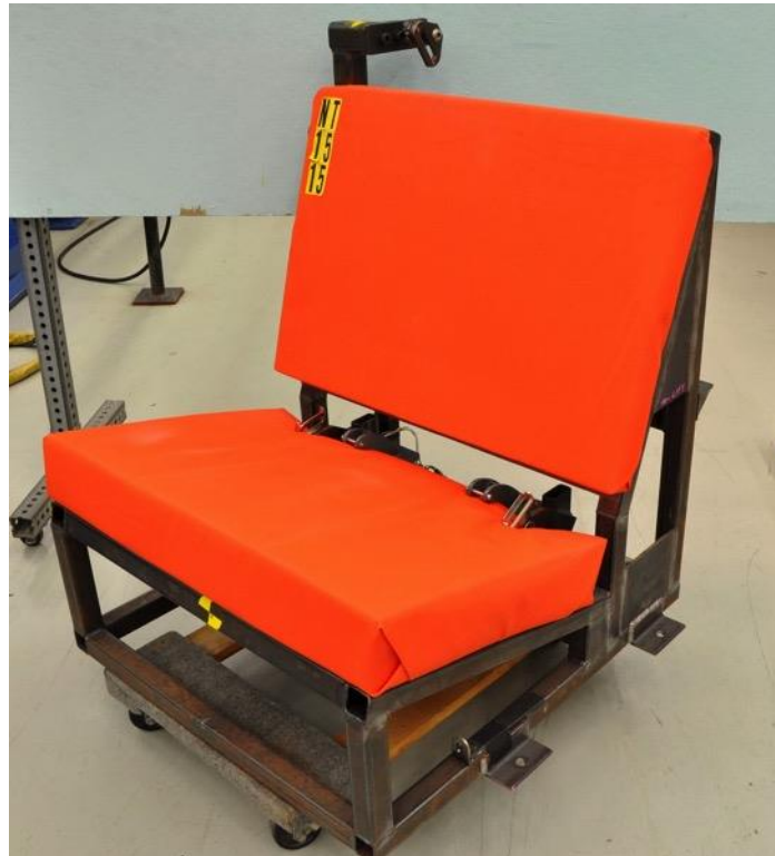
Figure 7. The preliminary 213 bench used for the test series.
