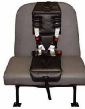
3. Put cushion in place and latch. Under the cushion, bring forward and connect the 1.5" strap to the front side buckle on front of seat (hold the pad on the seat).
