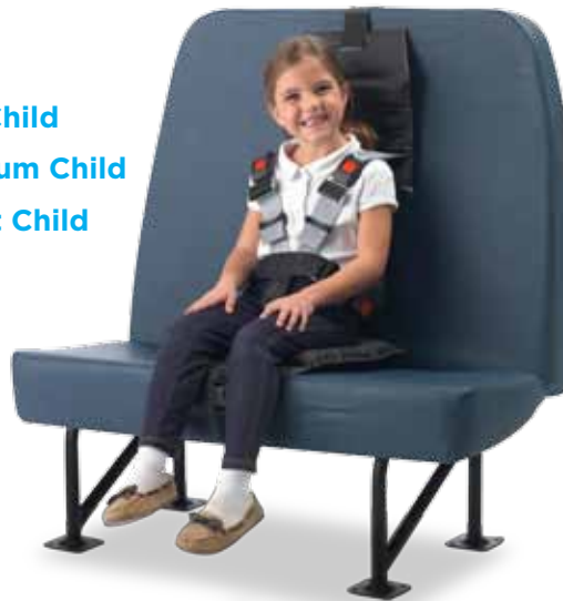
6. When using the Pro-Tech II place child in seat. Connect the color coded straps together. Pull the adjustment straps to fit firmly across the hip and shoulder areas. You should not be able to pinch up the webbing. (Pinch Test)
