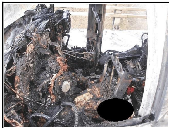
Figure 5. Interior damage front row, 2004 Chevrolet Silverado (police image)
