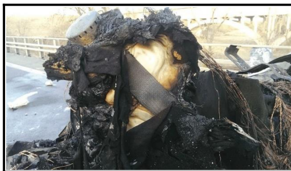
Figure 6. Driver's deployed frontal air bag, 2004 Chevrolet Silverado (police image)
