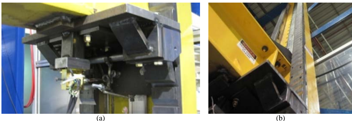
Figure 8-3. (a) Ratchet Catch Mechanism and (b) Vertical Ratchet Rails Mounted on Guide Beams
