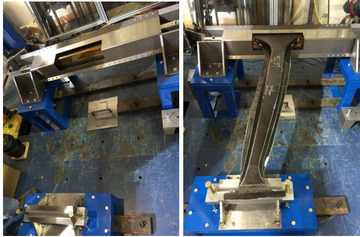
Figure 7-24. Assembled B-Pillar in Rocker Assembly and Impact Fixtures in Drop Tower
