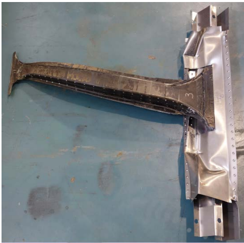
(a) Post-LVI Deformation and Damage
