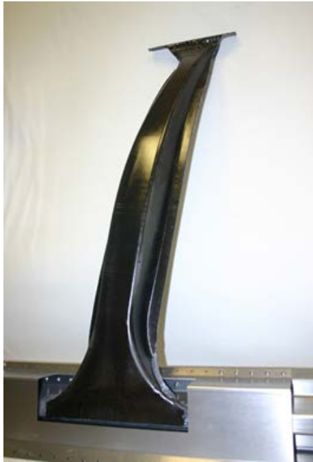
Figure 2-2. Adhesively Bonded Assembly of B-Pillar
