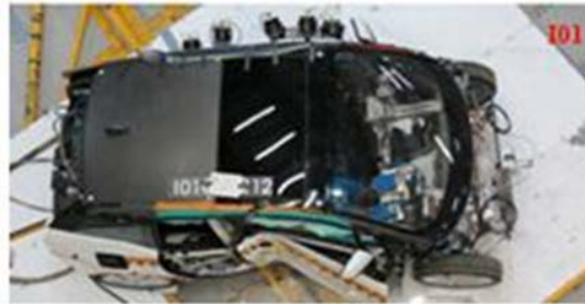
Figure 3-9. Occupant Compartment After Side-Impact, Steel (top) Versus CFRP (bottom)
