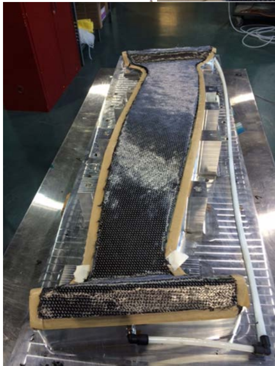
Figure 7-3. Preform Kitting and Assembly on Tool
