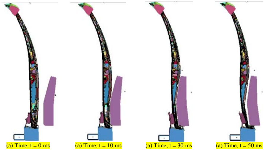
Figure 6-21. LS-DYNA Crash Simulation Result at Various Times Composite B-pillar design G50 computational run #90 designated by "091-G50." Material AS4/Nylon, Total Weight 7.26 kg as compared to Metal Baseline weight of 9 kg.
