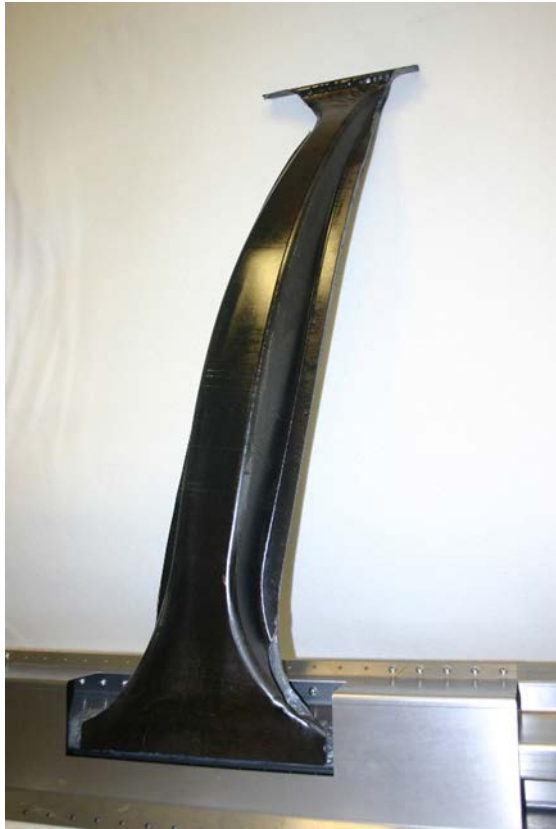
Figure 7-26. Adhesively Bonded Assembly of B-Pillar and Rocker
