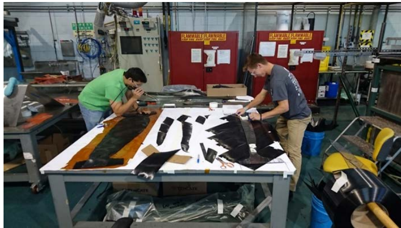
Figure 7-18. Assembly of Prepreg Pieces to Form Hat Blank
