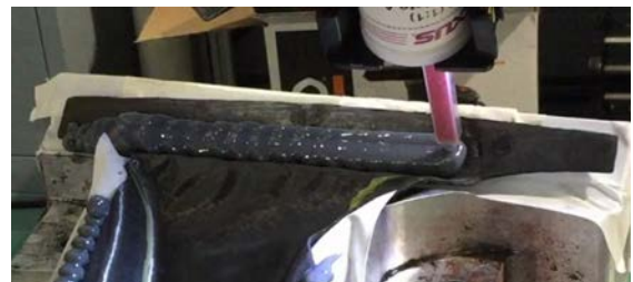
Figure 7-22. Adhesive Dispensing with Robot Head on Hat Prior to Assembly
