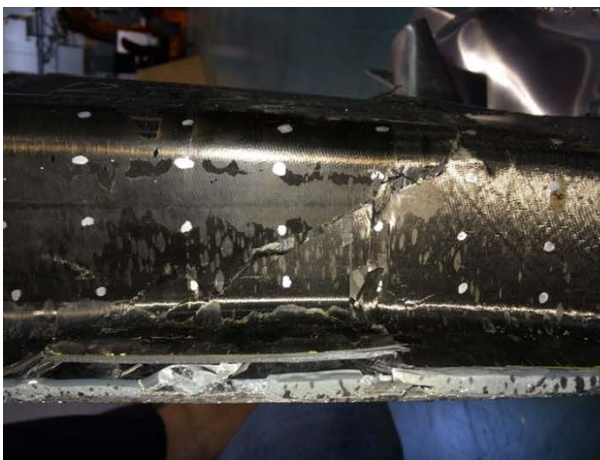
(c) Failure of the Hat and Spine Joint Region in the Crush Zone
