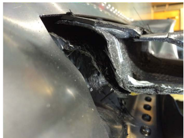
(d) Delamination of the Spine at the Rocker-Spine Adhesive Joint
