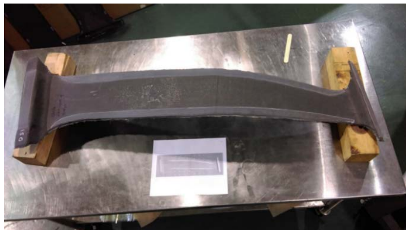
Figure 7-21. Surface Treated (grit-blast) Spine Section Ready for Assembly
