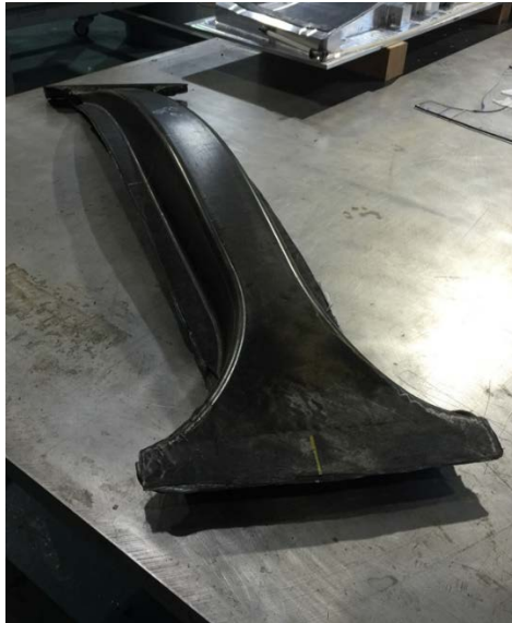
Figure 7-23. Adhesively Bonded Hat and Spine Assembly
