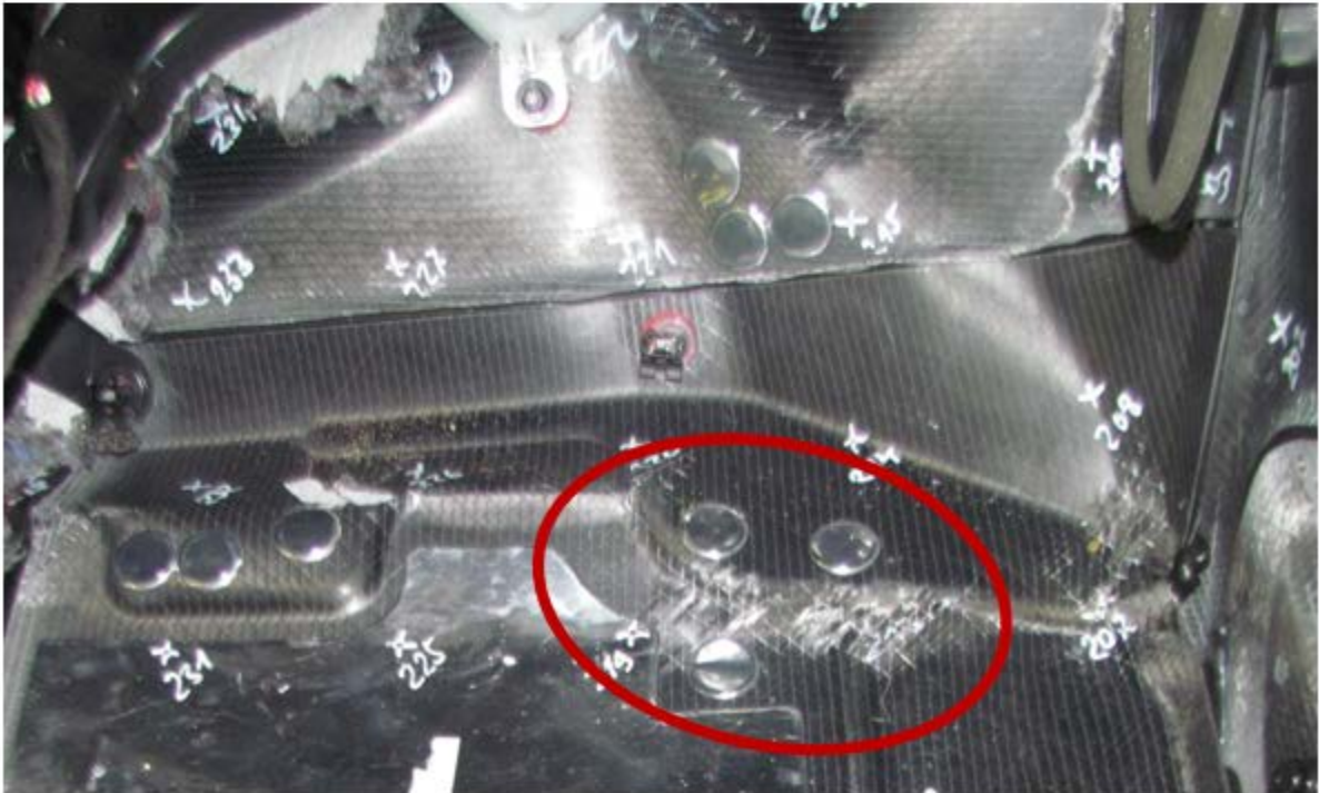
Figure 3-11. Footwell After Frontal Impact in CFRP Life-Cell With Lower (top) Versus Higher (bottom) Load Impact Energy
